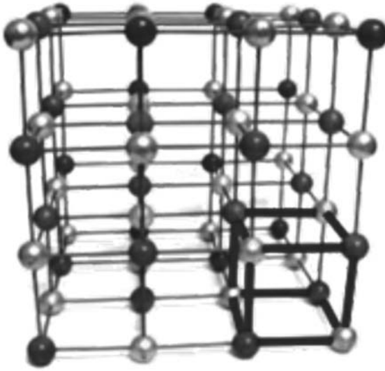
Figure 1.1 Arrangement of the sodium and chlorine atoms in the simple cubic lattice of sodium chloride.
